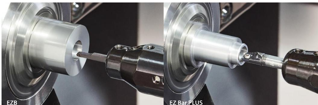
**EZ Bar and EZ Bar Plus multipurpose ID turning tools for small diameter**
